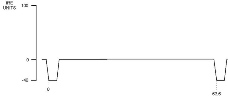
Figure 5-22 Transmitter Matrix Black Sync, 0 IRE, No Burst
